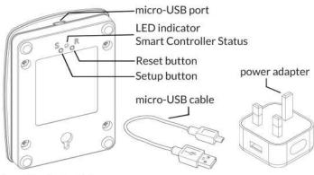
Smart Controller Status: Flashing blue - Hotspot available Flashing green - Connecting to the WiFi network Pulsing cyan/blue-green - Connected to the Internet
